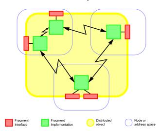
AspectIX distributed objects are fragmented over participating nodes or address spaces. The semantics of a distributed object are implemented by the entirety of its fragments. Therefore fragments communicate with one another. To interact with a distributed object, a client has a local fragment in its address space.
