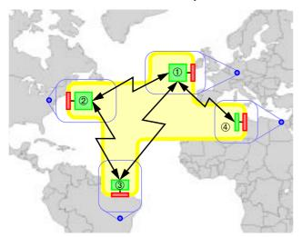
In a single distributed object, local fragments implementing strictly consistent replicas, ① and ②, can coexist with replicas having a looser consistency model like caches ③ or simple stubs ④. Fragments and consistency properties can change dynamically and transparently at run-time.
