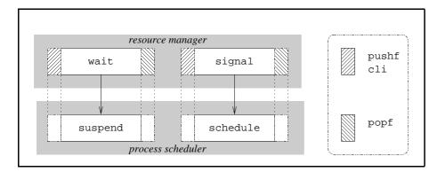
The critical sections of suspend() and schedule() are implicitly secured because both functions are called from within the already secured critical sections of wait() and signal(). Also note that, in this scenario, pushf could be deleted and popf could be replaced by sti. Any way, neither of these solutions is a good practice. Why?
