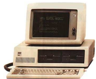
IBM PC model 5150, 1981 Intel 8088 PC-DOS (Microsoft) CP/M (Digital Research)
