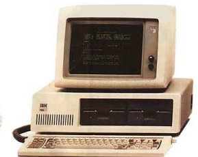
IBM PC model 5150, 1981 Intel 8088 PC-DOS (Microsoft) CP/M (Digital Research)
