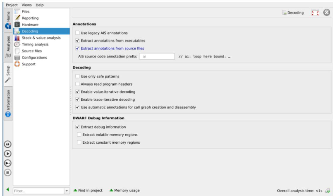
The screenshot shows the a<sup>3</sup> Analyzer software interface. The left sidebar contains a navigation menu with options: Home, Analyses, f(x), Setup, and Information. The 'Analyses' section is expanded, showing 'Decoding' as the selected tab. The main configuration area is divided into several sections:
