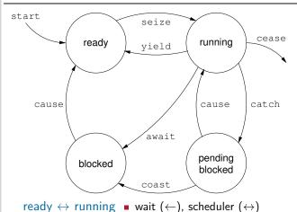
running → blocked ■ urgent wait blocked → ready ■ all, iff effective signalling (i.e., waiting signallee)
