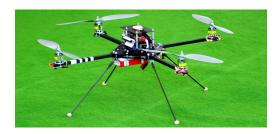
Fig. 3. The *14Copter* quadrotor helicopter; specifically designed with a redundant set of sensors.
