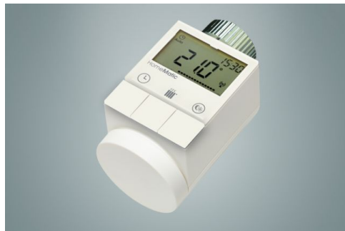
Figure 2.2: HomeMatic wireless radiator thermostat. The unit combines an actor for the radiator valve and a temperature sensor. Using a wireless connection target valve position or temperature can be set and the current temperature queried. Photo: Courtesy of eQ-3 AG
