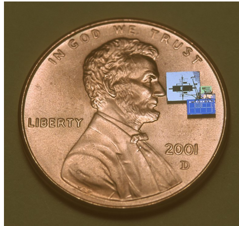
Figure 1.2: Mock-up of a 16\text{ mm}^3 solar powered smart dust mote with bi-directional communications. [War+02]
