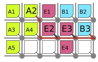
Figure 1: Tiled MPSoC system with running tasks from applications A, B and E. NoC communication (red, dotted) from task A2 to B3 needs to pass malicious tasks E2 and E3, where the malicious application E can eavesdrop and create frames.
