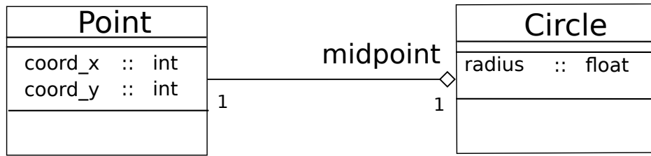
Figure 9: A simple class diagram which demonstrates a typical use case for inlining. The Circle class acts as a container object because its field reference radius holds a unique object.
