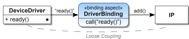
Figure 6: The principle of loose coupling. A binding aspect establishes a relation between two otherwise unrelated modules. The invocation of ready() is translated to an add() call, which registers the DeviceDriver at the IP stack.
